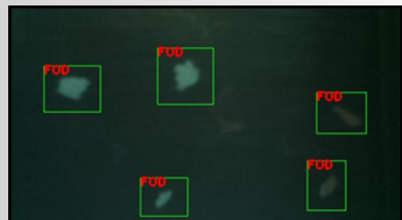
Foreign Object Detection with Color, Size, and Quantity Tata Advanced Systems Limited (TASL), Nagpur
